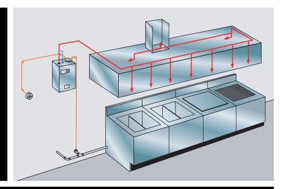
PRX<sup>™</sup> LIQUID FIRE SUPPRESSANT ■ OVERLAPPING PROTECTION HYBRID DUAL-AGENT CONCEPT ■ TWO BASIC DESIGNS WITH PROVEN FUSIBLE-LINK DETECTION AND RELEASE SYSTEMS ■ STAINLESS STEEL ENCLOSURES APPROVED AND LISTED UL300 AND 2092; ULC C1254.6; ASSE 1001; AND IAPMO PS108-98 ■ FIVE-YEAR LIMITED WARRANTY ANSUL K-GUARD<sub>8</sub> EXTINGUISHER FOR MANUAL BACKUP
