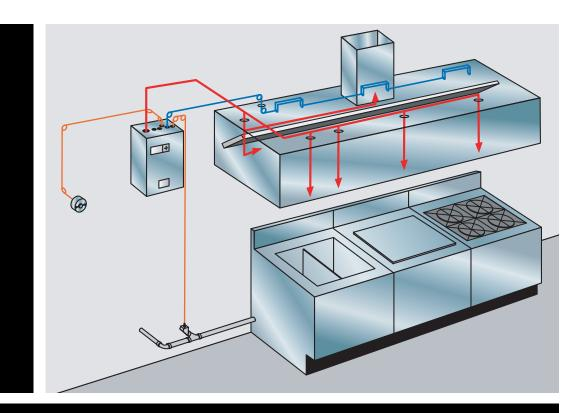
ANSULEX: LIQUID FIRE SUPPRESSANT TWO BASIC DESIGNS WITH PROVEN FUSIBLE-LINK DETECTION AND RELEASE SYSTEMS STAINLESS STEEL ENCLOSURES UL300, ULC, MEA, ABS AND CE APPROVED AND LISTED,
